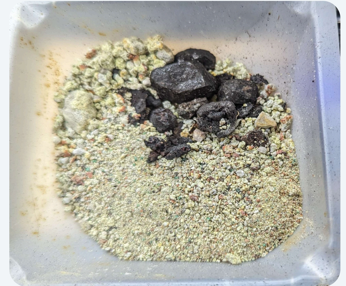
Recovered rare earth oxide concentrate from a continuous mining unit run, before refining.
