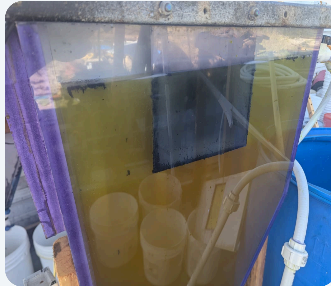
A running cell: leach liquor and the deposit forming.
